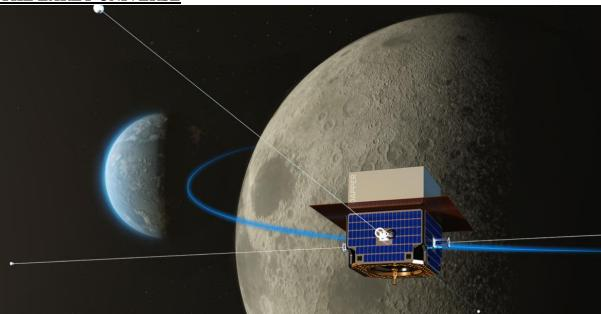
Artist illustration of the Dark Ages Polarimetry Pathfinder (DAPPER), which will look for faint radio signals from the early universe while operating in a low lunar orbit. Its specialized radio receiver and high-frequency antenna are currently being developed by NRAO. Credit: NRAO/AUI/NSF, Sophia Dagnello
